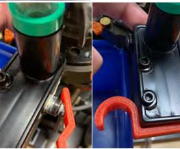
5. To store the Case Feed Stop when not in use simply snap the round part on the Casefeed Tube.
