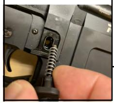
Remove the stock spring and slide the new spring over the screw. Direction does not matter but you will notice that the new spring is shorter than the stock spring. I suggest that you use a little light grease or thick oil on the oval section of the mag release button that fits in the oval cutout in the receiver.
